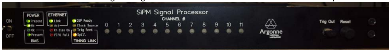
Figure 7 - Front panel of SSP after programming of FPGAs
